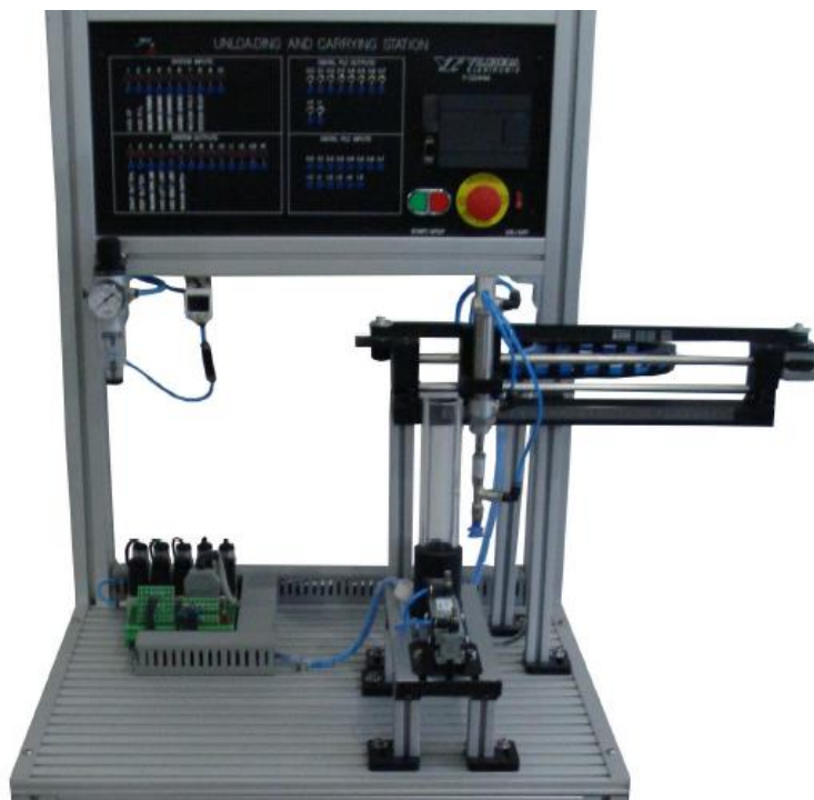
Figure 6.1 Unloading and Carrying Station [13]
