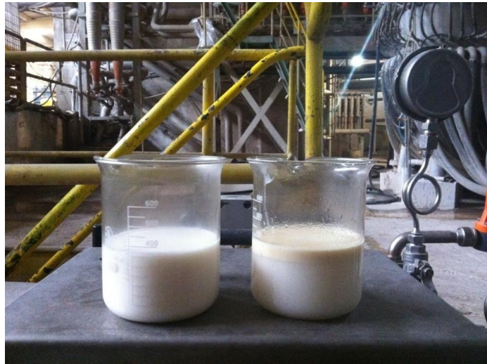
Figure 4.17 : Non-homogenous or yellowish emulsion. Emulsion on the left side is correct.
