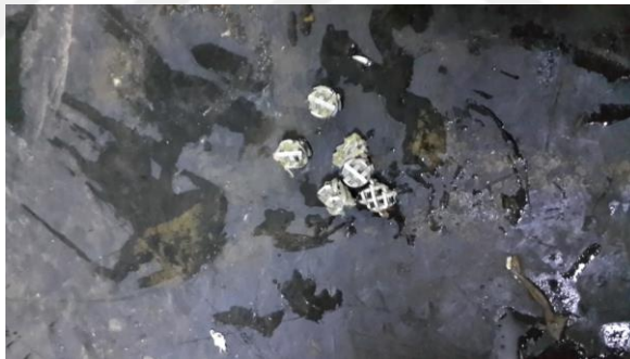
Figure 4.15 : 6 mixing elements under the ring disc
