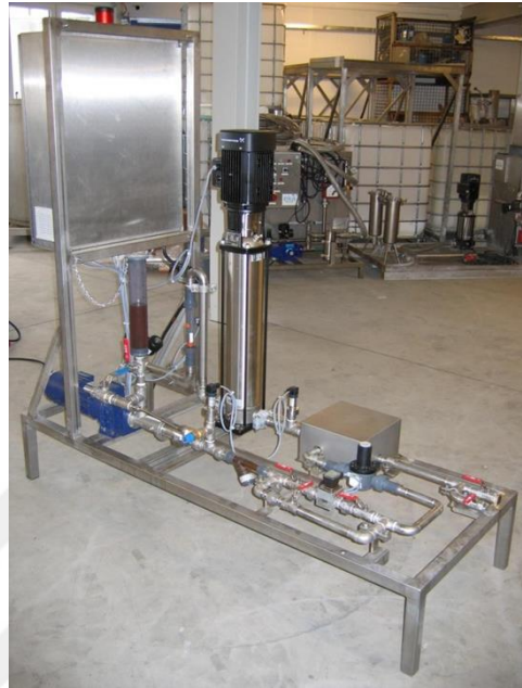
Figure 3.1 : Turbine system industrial ASA emulsification
