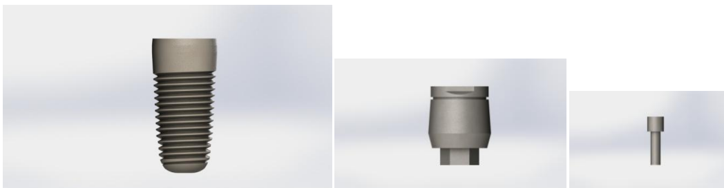
Şekil 3-5: 3D 4.7 mm Tapered Screw-Vent implant, HLA 5/6 abutment ve vida modeli
