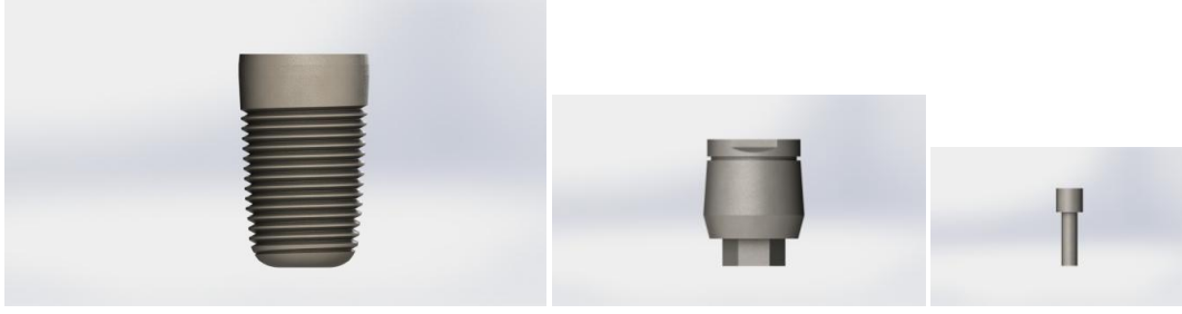
Şekil 3-6: 3D 6.0 mm Tapered Screw-Vent implant, HLA 5/6 abutment ve vida modeli
