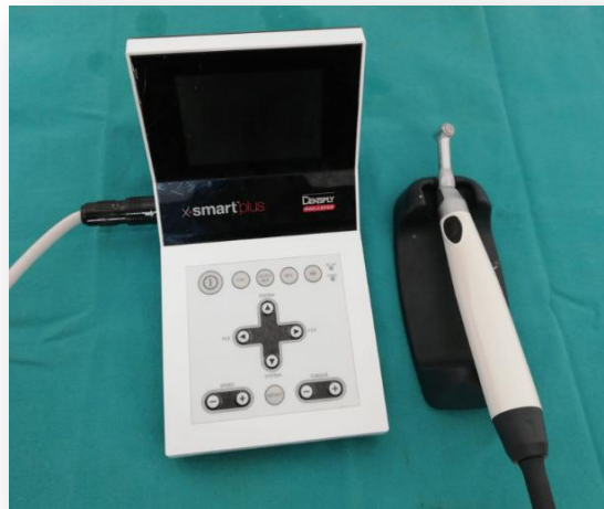
Resim 12. X-Smart Plus endodontik motor
