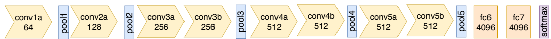
Figure 2.1: 3D Convolutional Neural Network (C3D) [4] architecture with 8 convolutional, 5 pooling and 2 fully connected layers.
