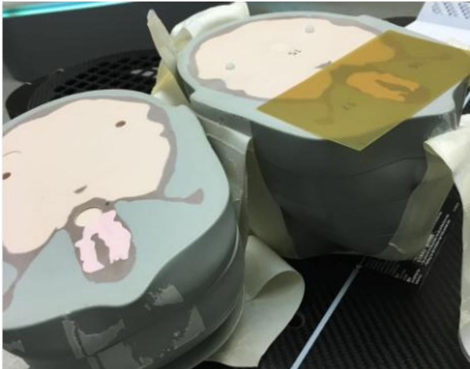
Photo 5.2.8.2.Position of film on nasal cavity part of Phantom
