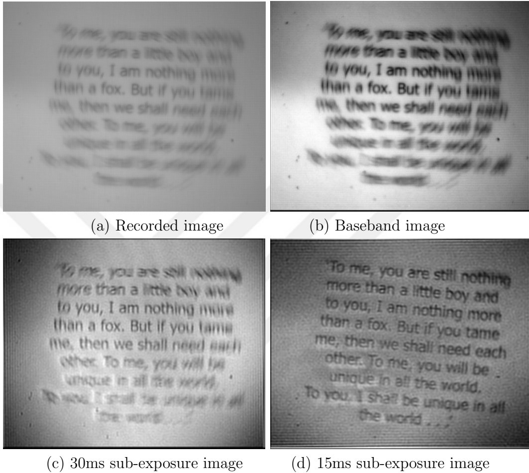
Figure 4.8: FDMI experiment with the prototype system - Moving planar surface.
