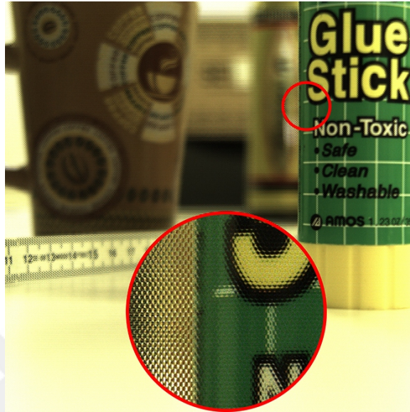
Figure 3.1: A lenslet image downloaded from a first generation Lytro camera.
