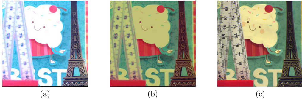
Figure 4.4: Photometric registration of light field images and regular sensor image. (a) Middle sub-aperture light field image before photometric registration; (b) Middle sub-aperture light field image after photometric registration; (c) Homographically corrected image from regular sensor taken as the reference for photometric registration.
