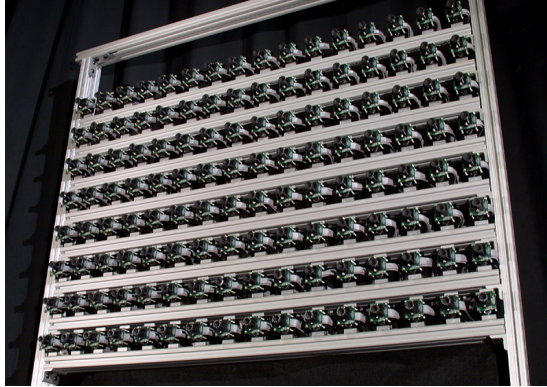
Figure 2.3: Camera array of 8x16 cameras to create light field developed by Stanford [1].
