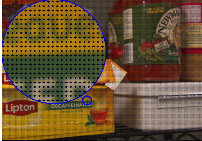
Figure 3.1: Light field captured by a Lytro Illum camera. A zoomed-in region is overlaid to show the individual lenslet regions.
