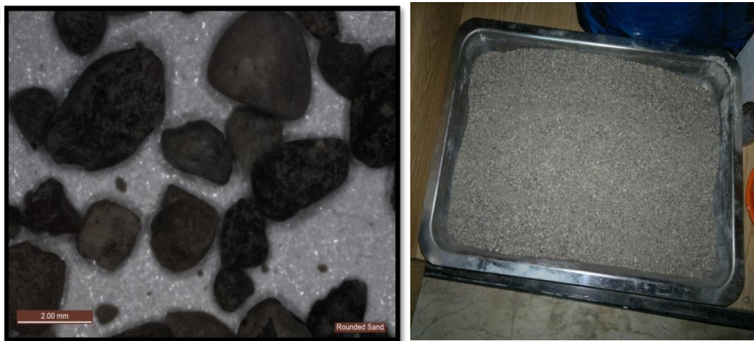
Figure 3.2: River sand particles used in the testing program (Electronic Microscope)
