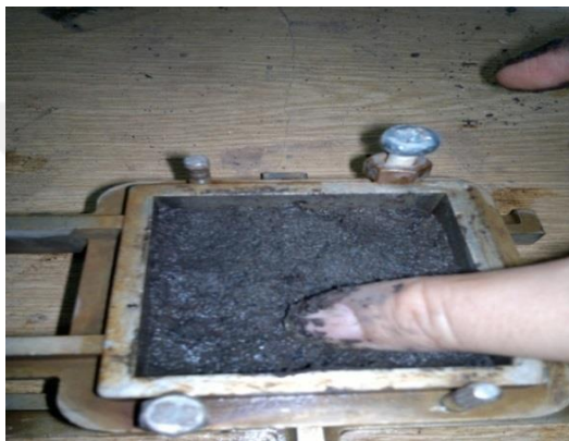
C21: Preparing samples for direct shear test
