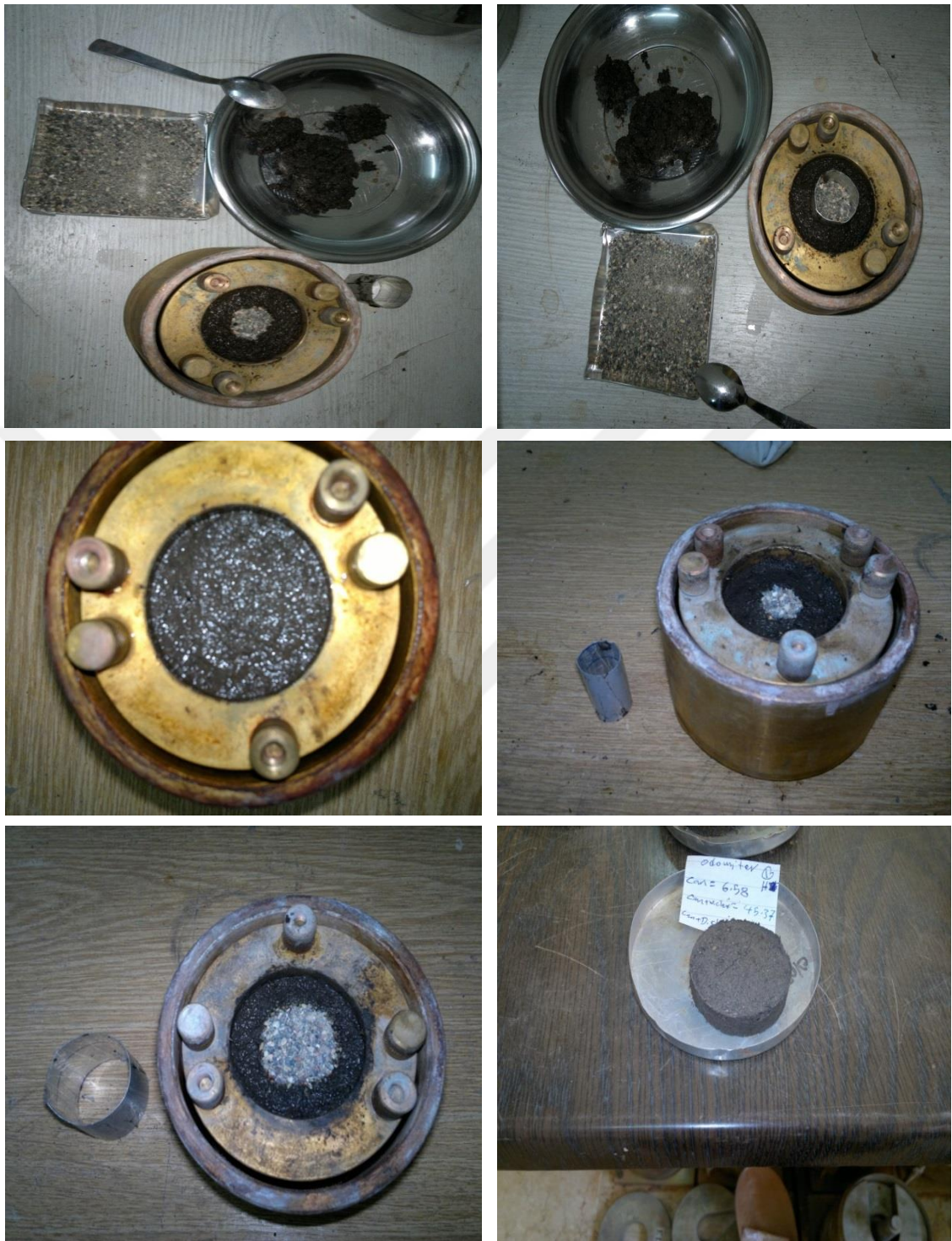
Figure 3.8: Steps for sample preparation for consolidation test
