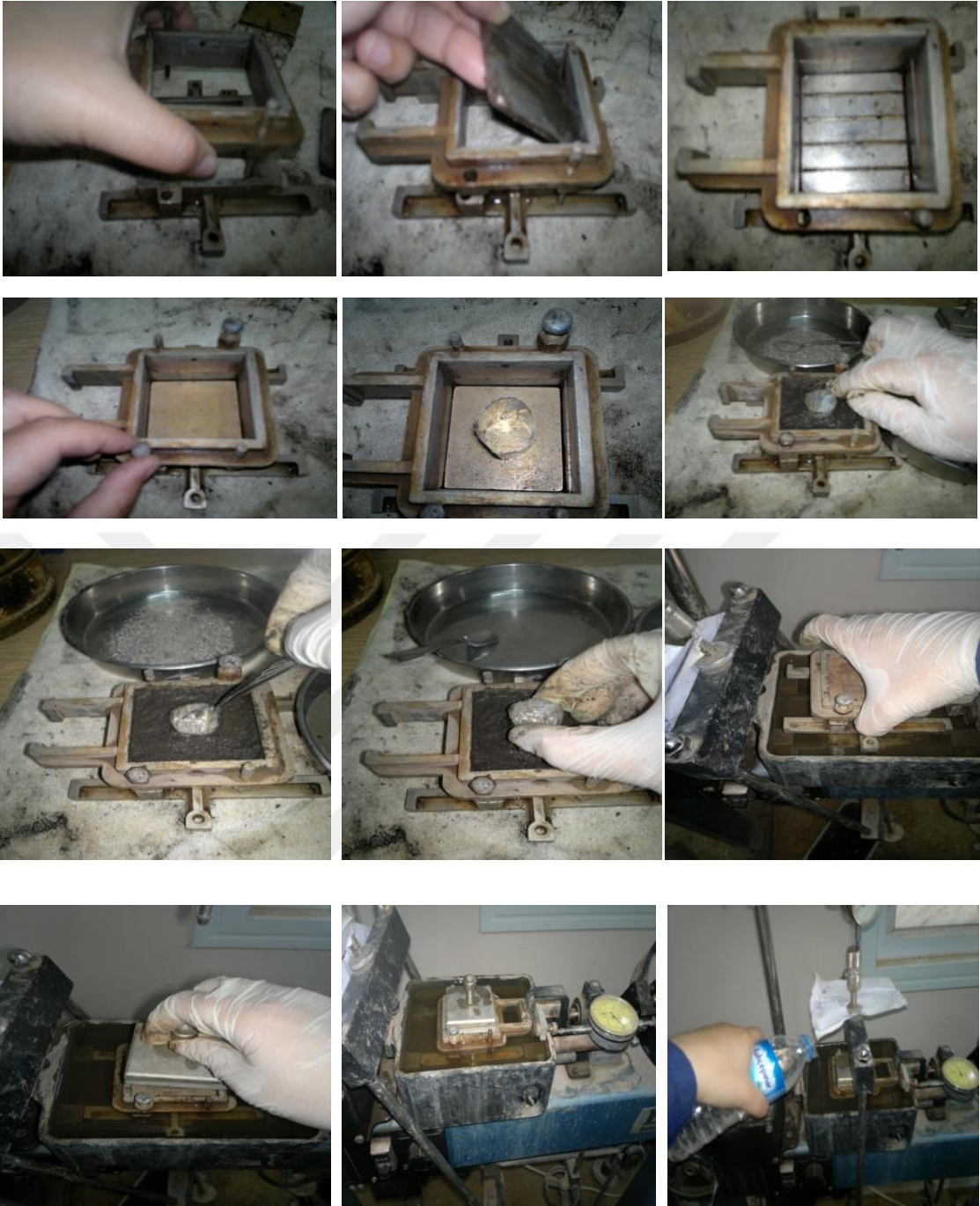
Figure 3.10: All procedures of direct shear test
