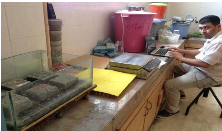
Figure B 2 Photographic view during concrete sorptivity test
