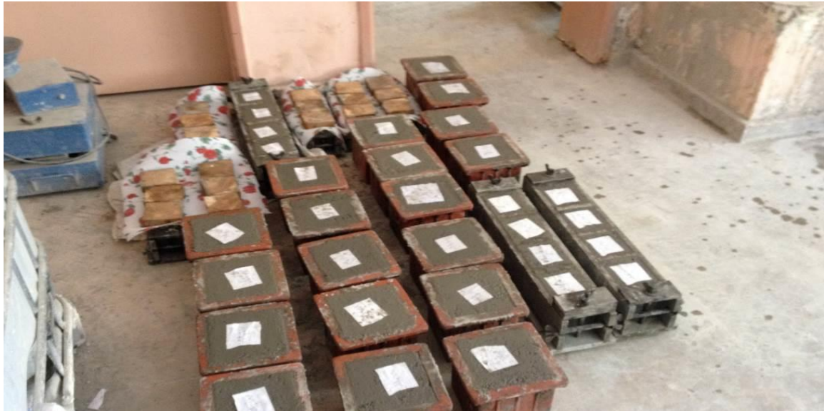
Figure B 3 Photographic view of molded specimens
