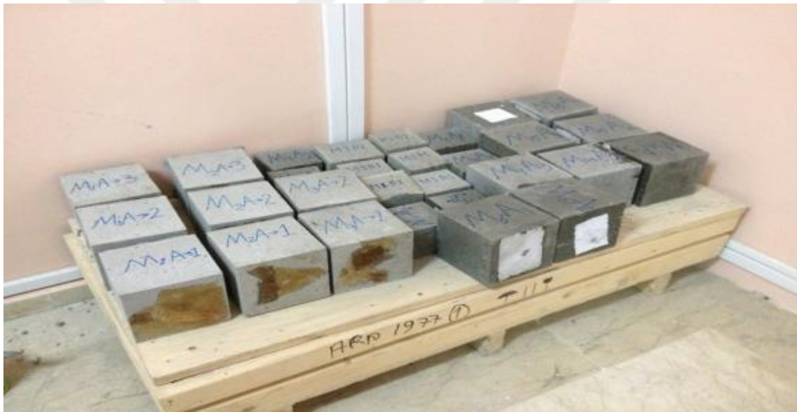
Figure B 4 Photographic view of demoulded specimens during air curing.
