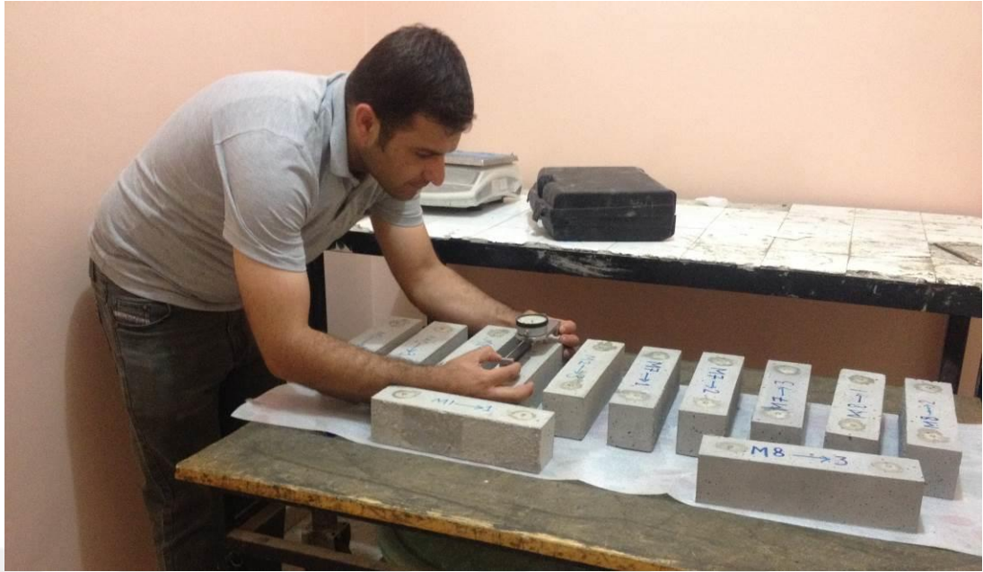
Figure B 5 Photographic view of shrinkage reading by dial comparator
