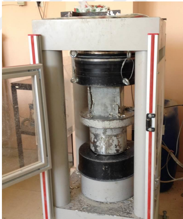
Figure B 6 Photographic view of compressive strength testing
