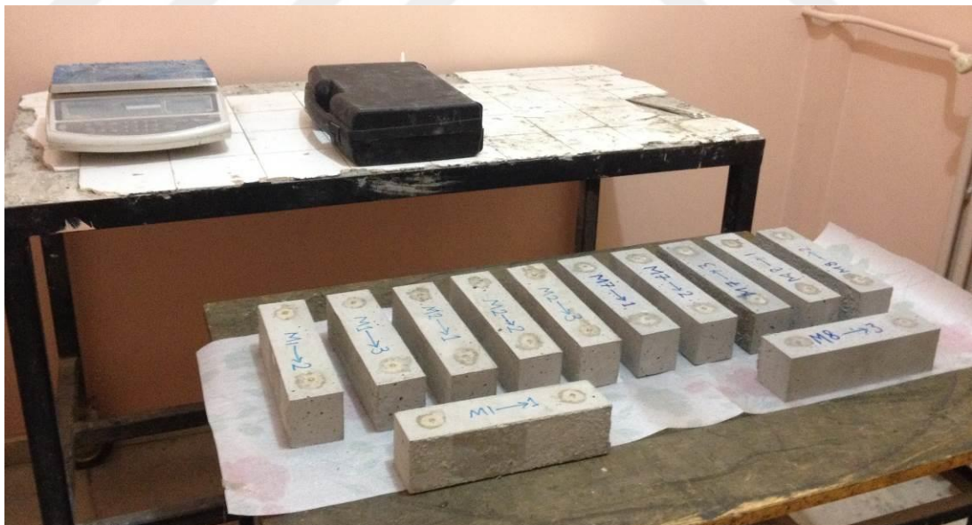
Figure B 4 Photographic view of shrinkage specimens and curing room (controlled temperature and humidity)
