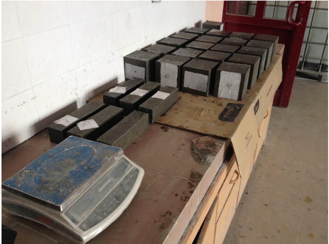
Figure B 3 Photographic view of demoulded specimens
