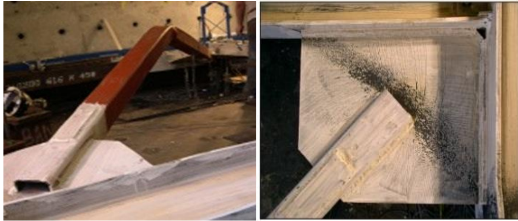
a) Brace buckling deformation
