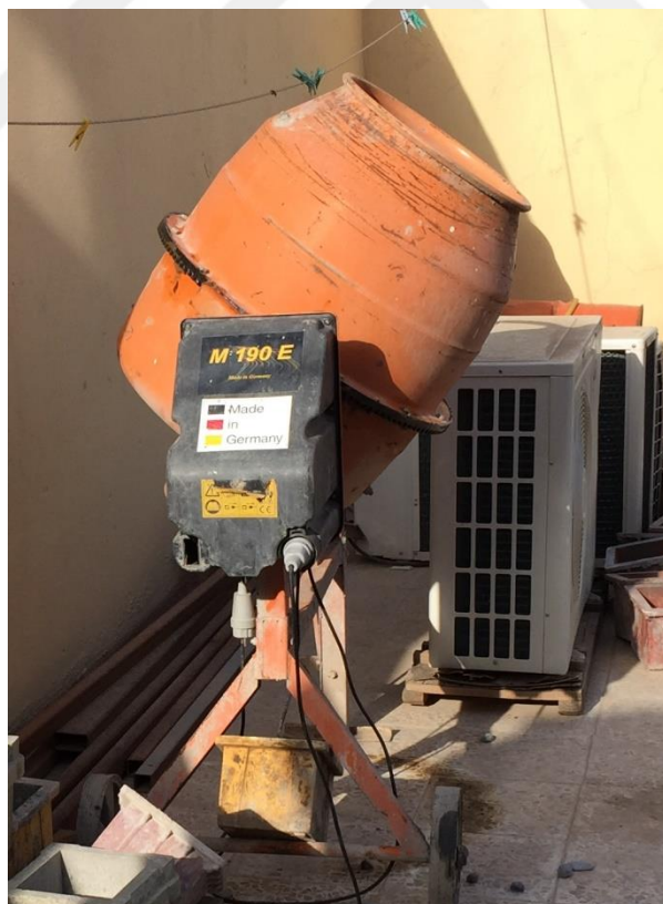
Fig (3.5) the electric mixer of concrete was used
