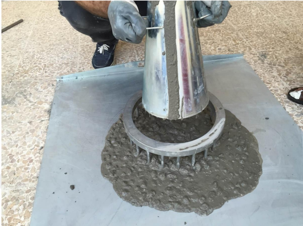
Fig (3.12) j-ring test
