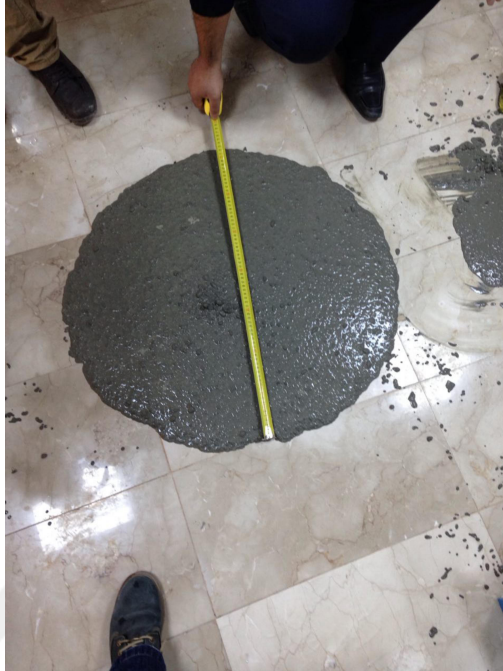
Figure 3.3: Measurement of slump flow diameter
