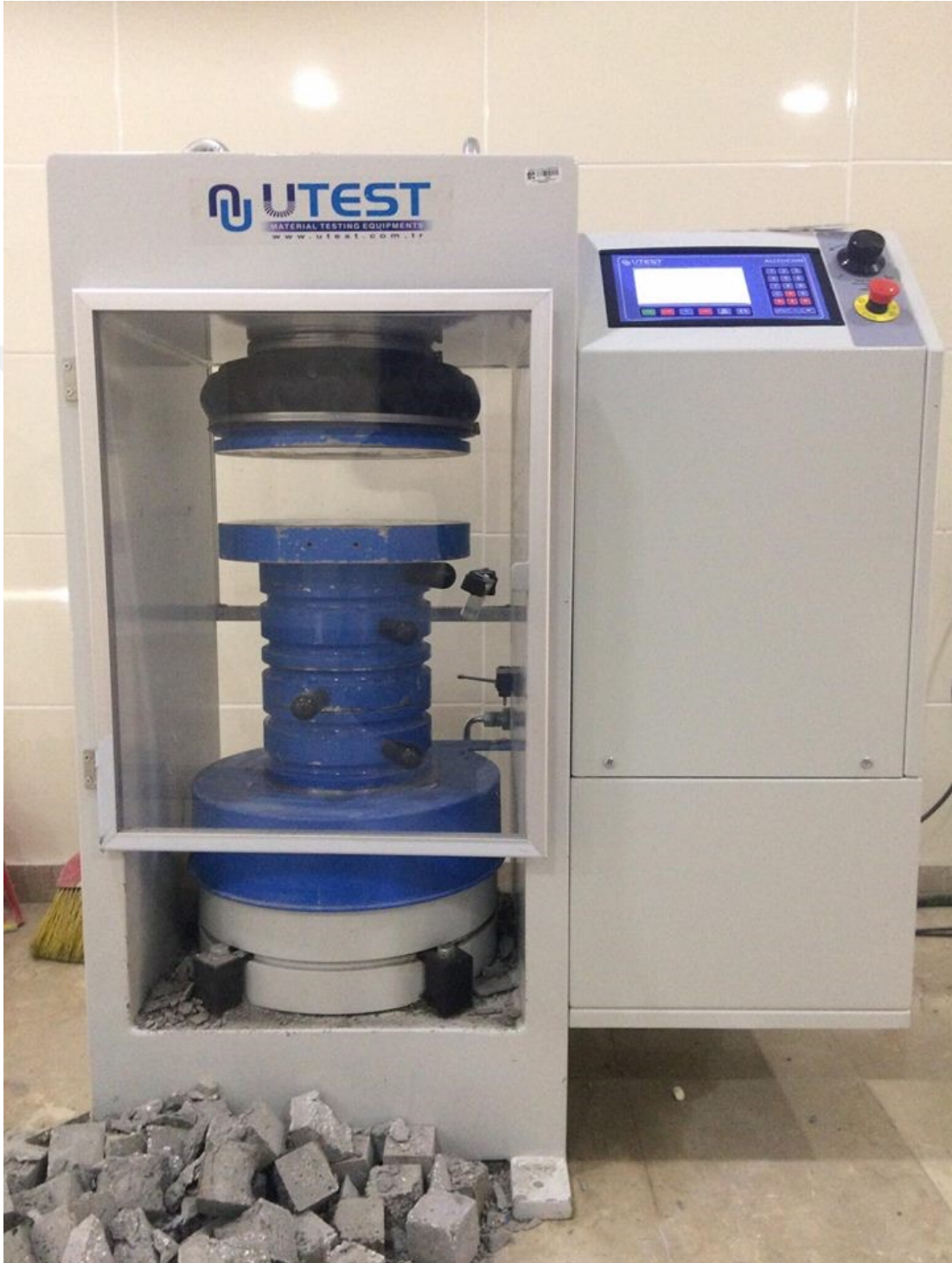
Figure C 4 Photographic view of compressive strength testing
