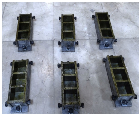
Figure 3.6 Preparation of mortar and casting
