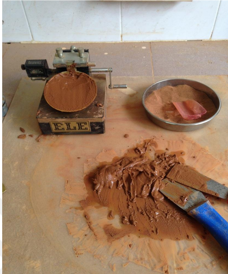
Figure 3.14 Samples prepared for liquid limit test
