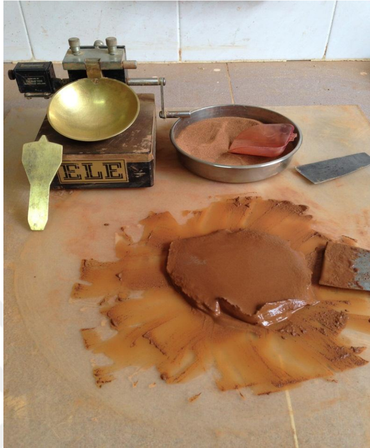
Figure 3.13 Preparation for the LL, PL and PI tests
