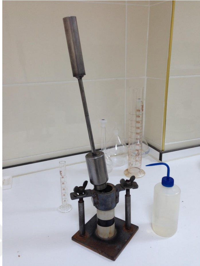
Figure 3.10 The compaction hammer and the plastic split mold used for UCS test
