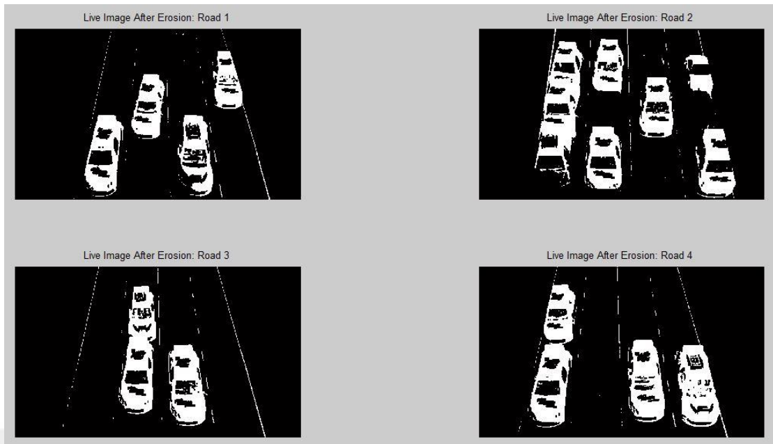
Figure 4.15 Live image after erosion operation (structure element: square, size: 4)
