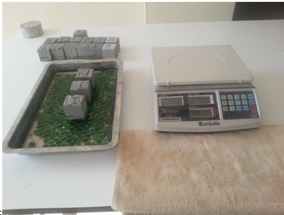
Figure 3.16 Sorptivity test setup.
