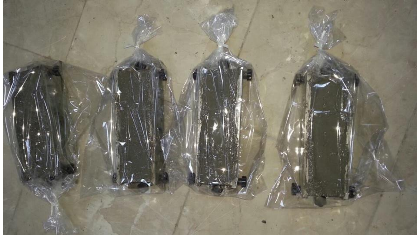
Figure 3.10 Mortar sealing with a heat resistant film.
