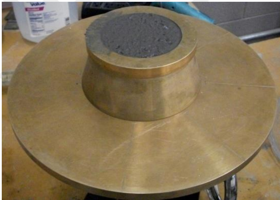
Figure 3.13 Flow table test apparatuses.
