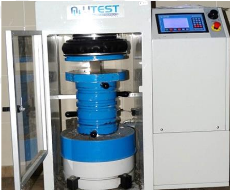
Figure 3.12 Mortar cube compressive strength test.
