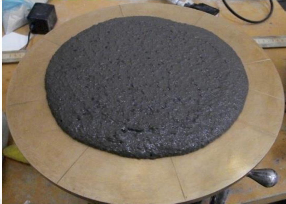
Figure 3.14 Photographic view of mortar flow.
