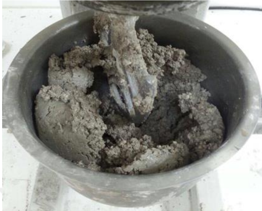
Figure 6.1 Hardened LWGM during mixing in mixer.
