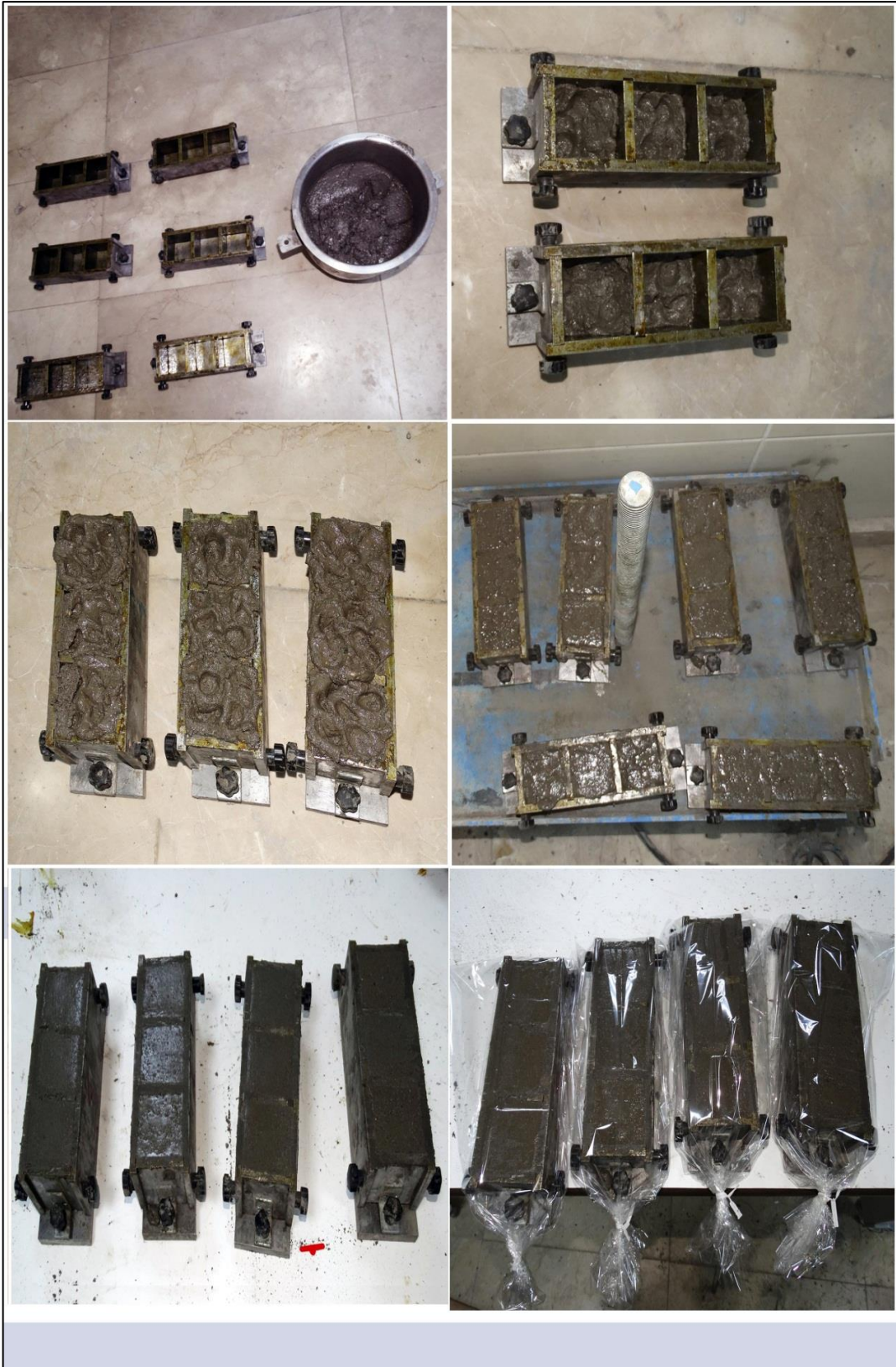
Figure 3.4 Casting geopolymer mortars
