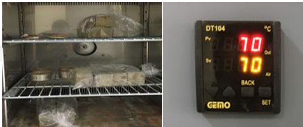
Figure 3.5 Dry (oven) Curing
