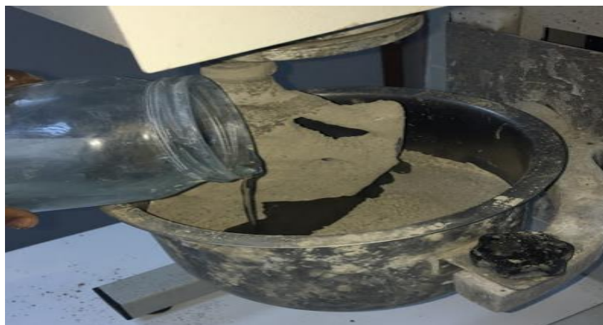
Figure 3.3 Adding alkaline activator to the dry components
