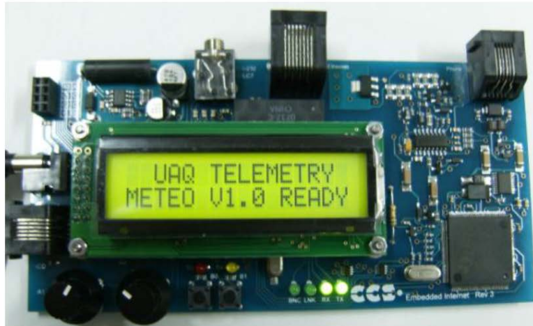
Figure 2.24: Embedded HTTP Server, implemented by M. Toledano-Ayala and others 2011, [51].
