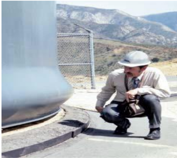
Figure 2.1 Elephant foot buckling (Anumod, et al., 2014)
