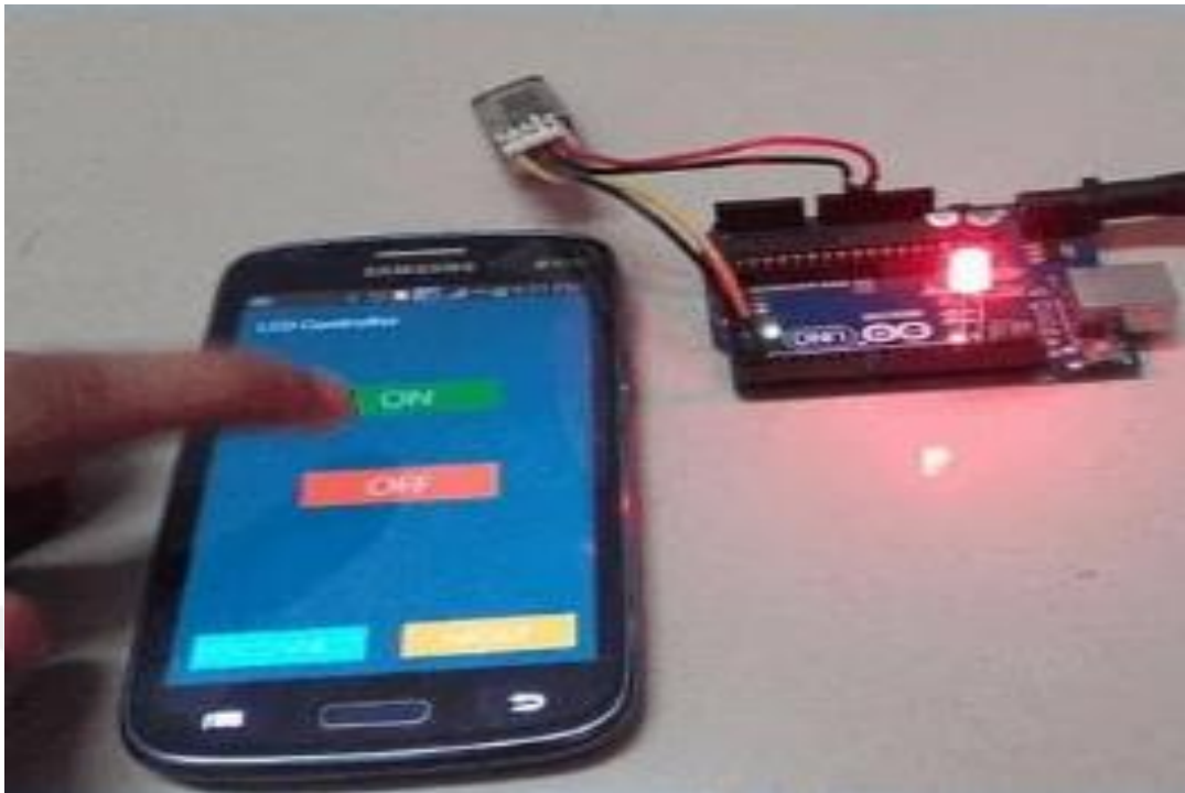
Figure 31. Implementation of home appliance control via Bluetooth
