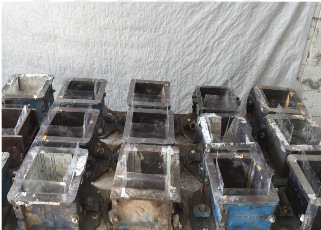
Figure A-8 Putting PVC cover to cubes
