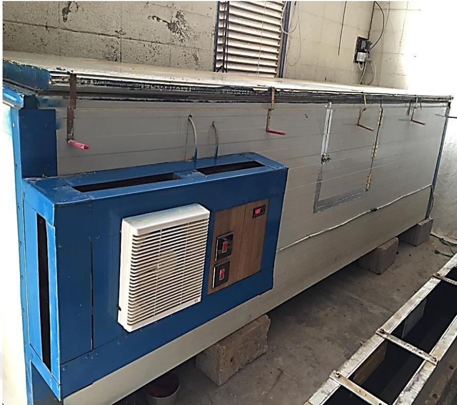
Figure A-13 Dry oven (1*1*4) meter
