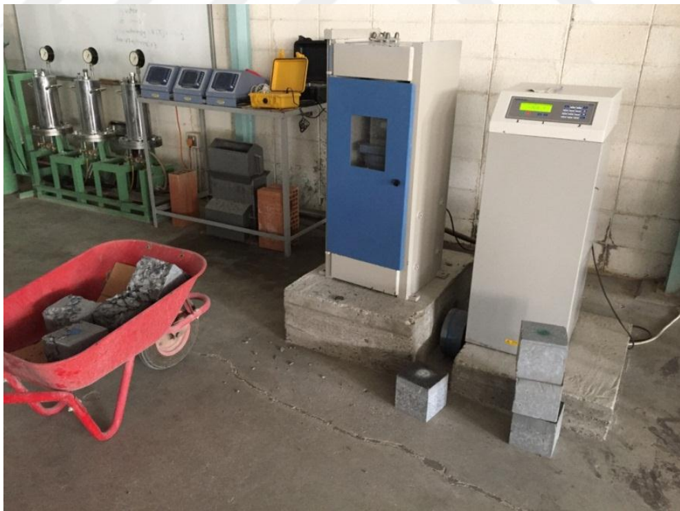
Figure B-2 Compressive Strength test for geopolymer concrete cubes
