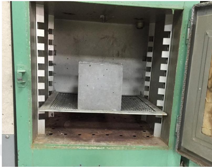
Figure 3.12 Arrangement of specimens in the oven
