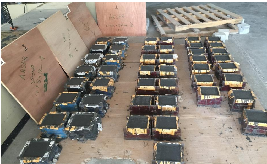
Figure A-12 Rest period after casting to (24) hour
