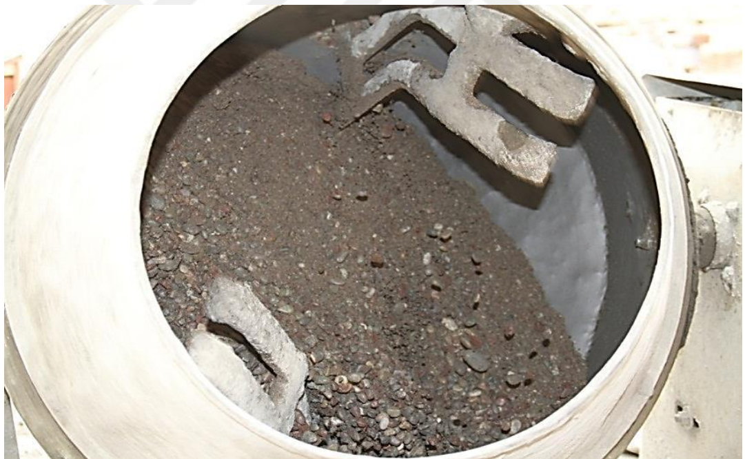
Figure A-4 Pan mixer without alkaline solution
