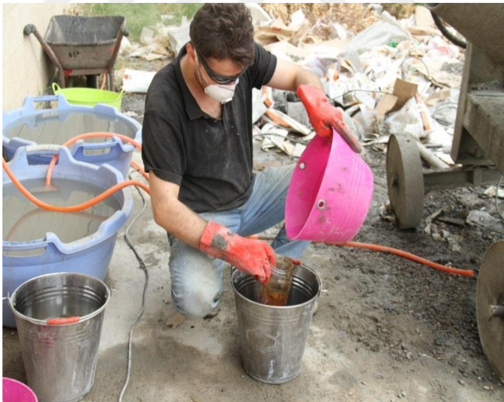
Figure A-6 Super plasticizer mixed with remaining extra water
