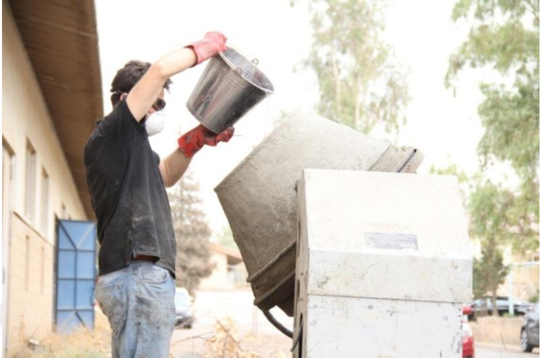
Figure A-5 The alkaline liquid was mixed with dry mixture
