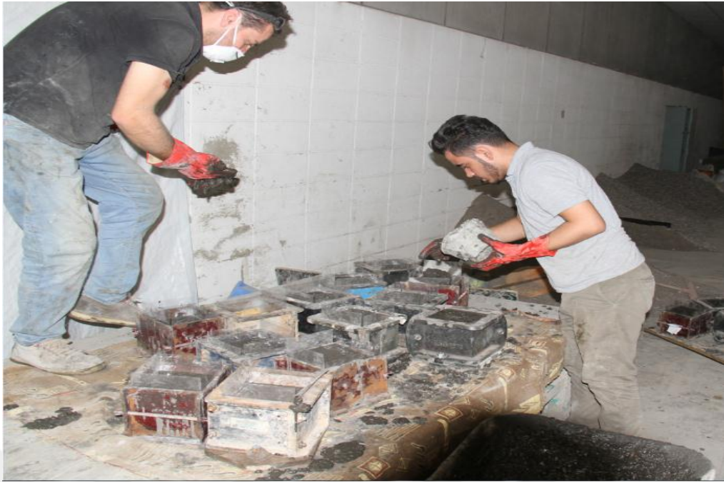
Figure A-9 Casting cubs on the vibrator
