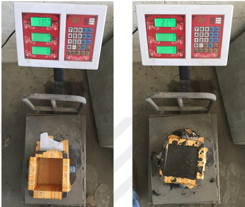
Figure 3.11 Weight measurements for density calculation
