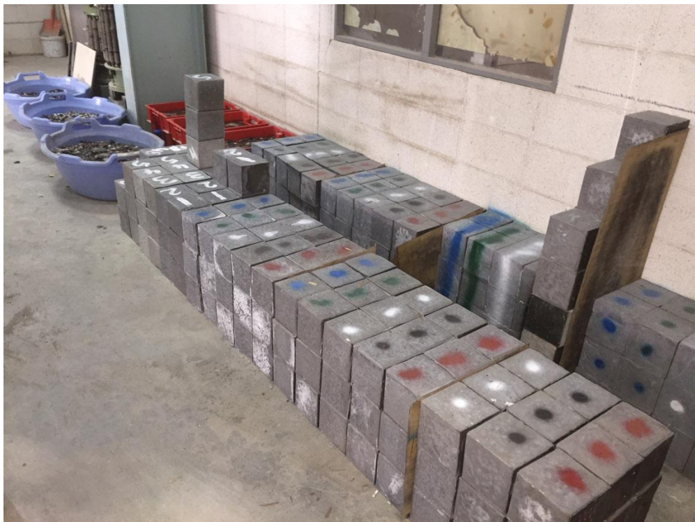
Figure 3.2 After casting geopolymer concrete cubes
