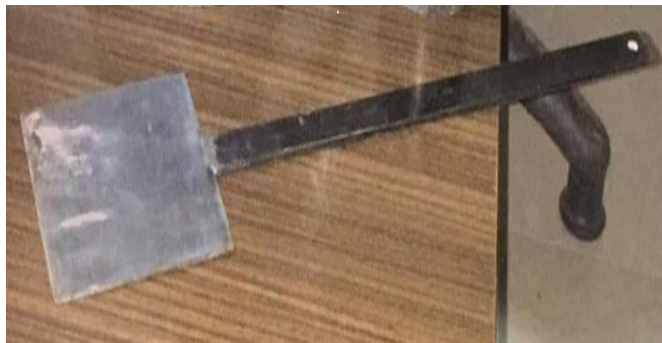
Figure 5. 6: Plate cohesion test apparatus
