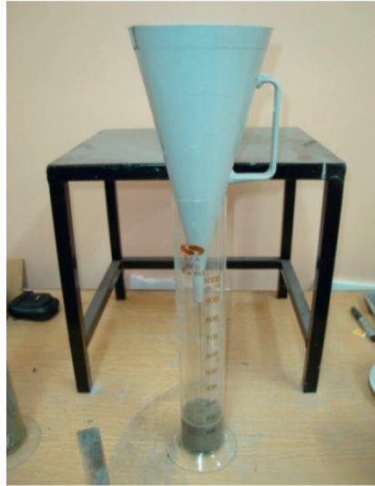
Figure 5. 5: Marsh cone flow test apparatus
