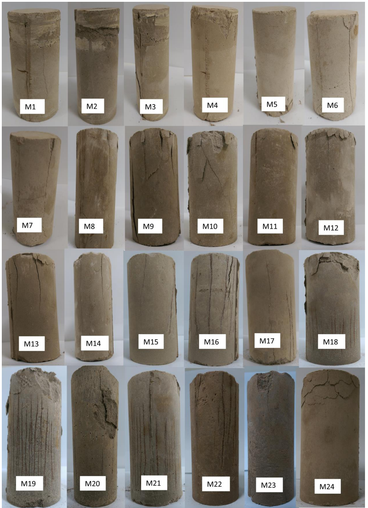
Figure 6. 28: Failure criteria of the soilcretes samples for 28 day curing. (WMP)
