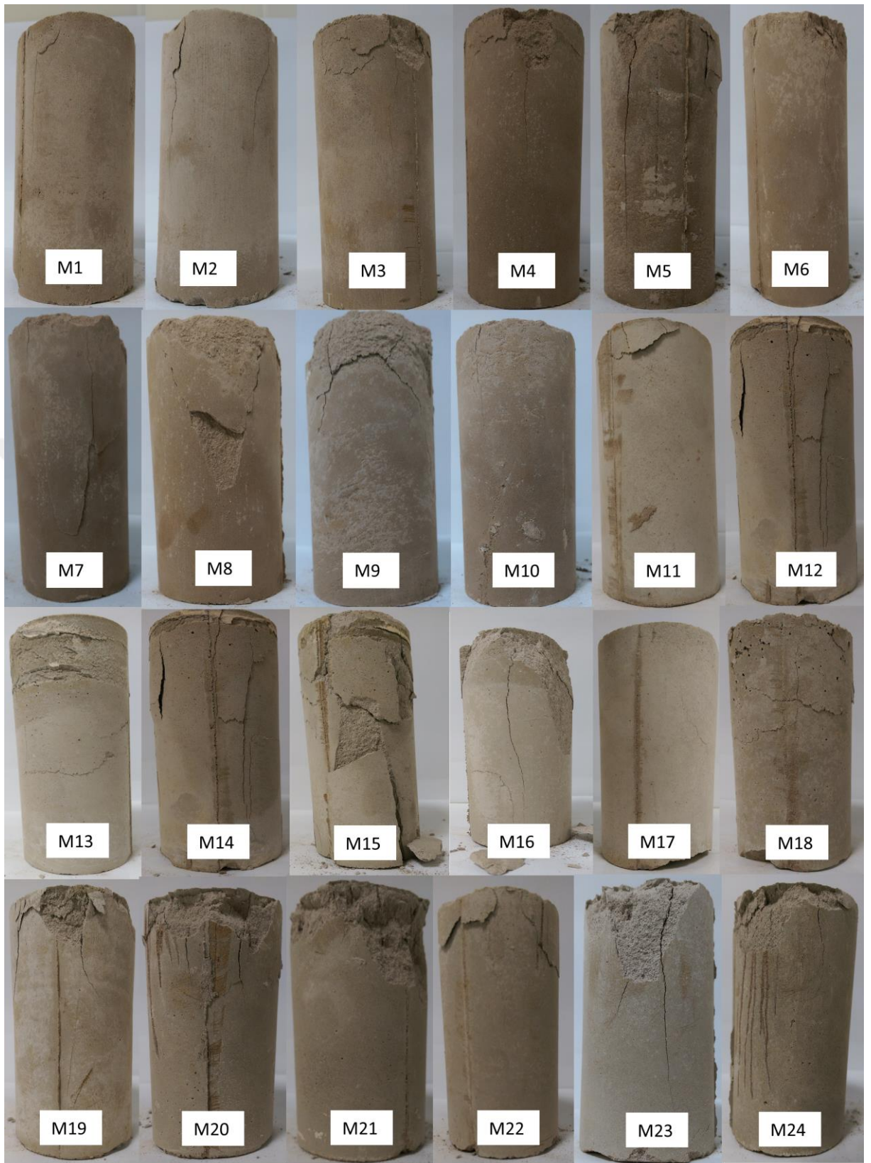
Figure 6. 29: Failure criteria of the soilcretes samples for 28 day curing (WMP+FA)
