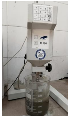
Figure 4. 4: Rotational viscometer (Rheometer)
