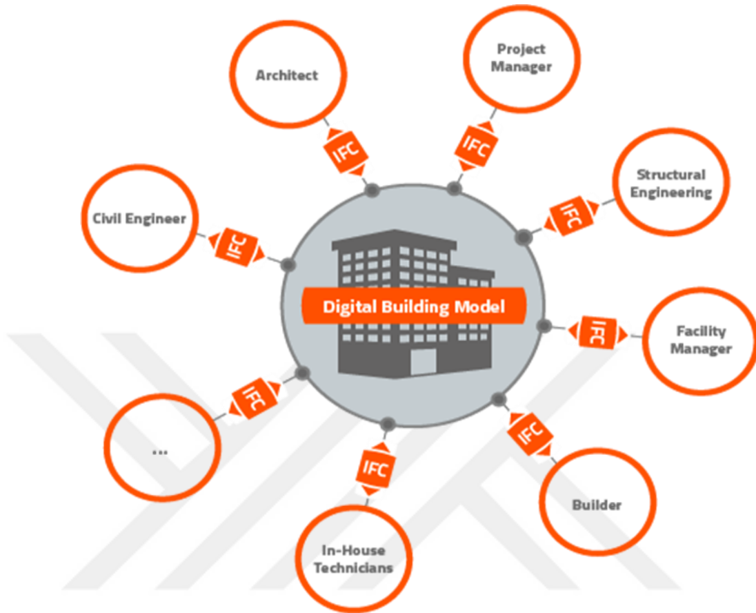
Figure 31: BIM Information Exchange Management
