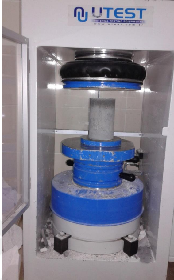
Figure 4.3 Concrete sample in UCS test
