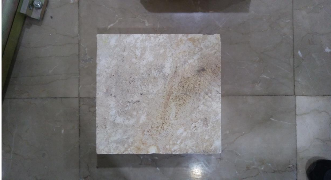
Figure 3.3 Two adjacent limestone blocks (15×30×15 cm)
