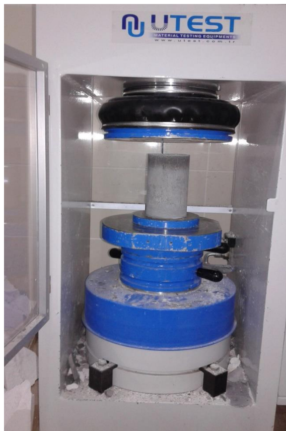
Figure 3.11 Uniaxial compression test of infilled concrete sample
