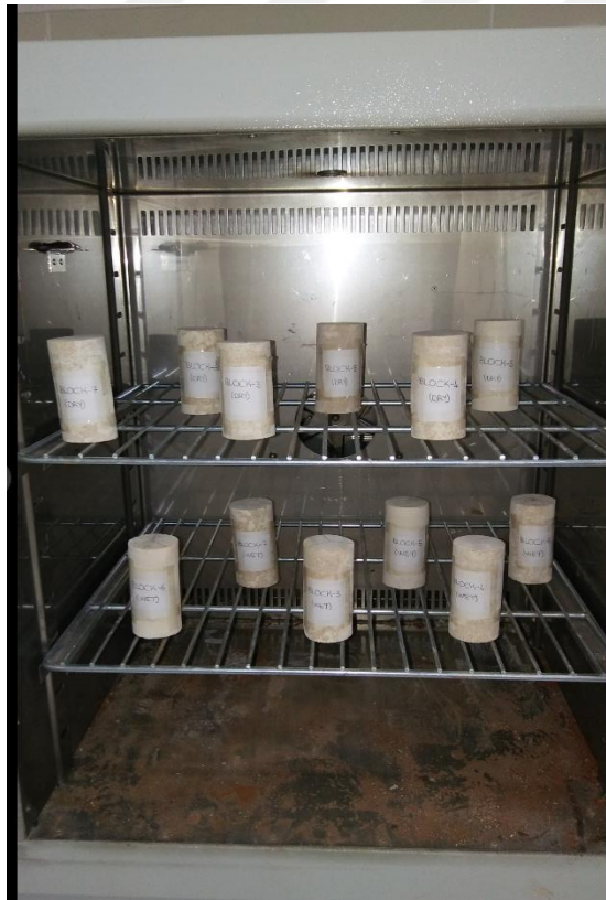
Figure 3.7 Drying of the cylindrical samples in the laboratory oven
