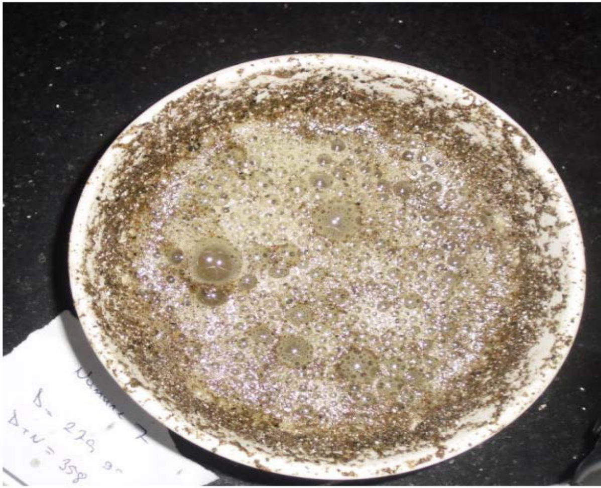
Photo 128 . As a result of acid treatment of sample number 7
