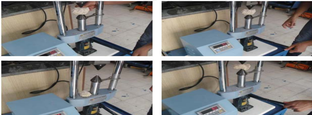
Photo 123 . Specimens subjected to point load test in laboratory environment
