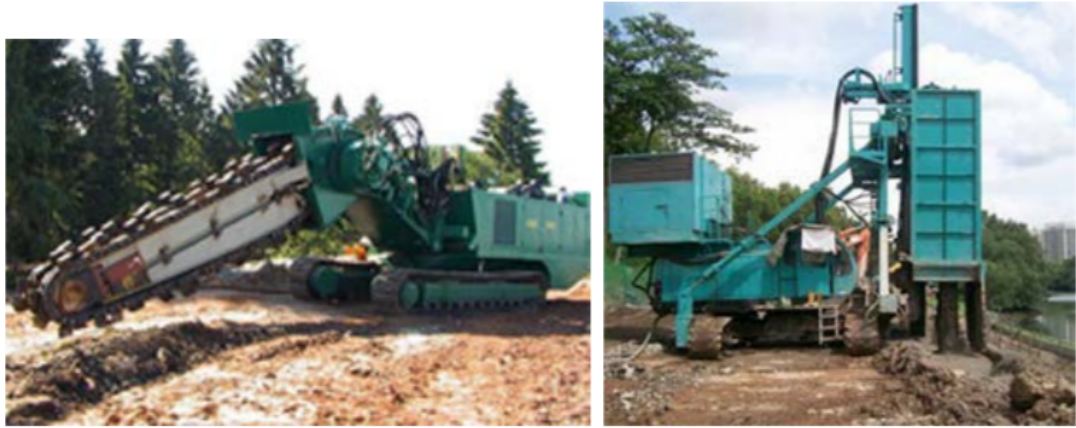
Figure 2.5: The FMI and TRD–Trenching machine for construction of deep walls (Massarsch and Topolnicki, 2005)
