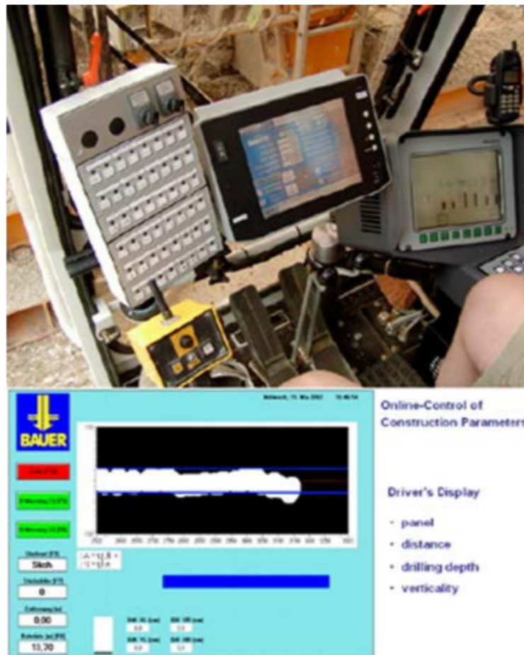
Figure 2.13: Online quality control/quality assurance of construction parameters (Stocker and Seidel, 2005)
