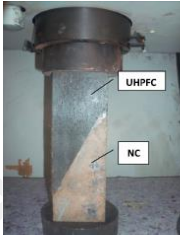
Figure 2.3. Slant shear test set-up for the composite concrete specimen (Tayeh et al., 2012)
