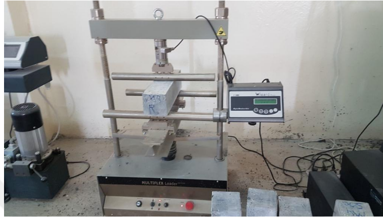
Figure 3.16. Test setup for flexural strength
