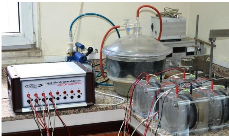
Figure 3.22. Rapid chloride permeability test set-up
