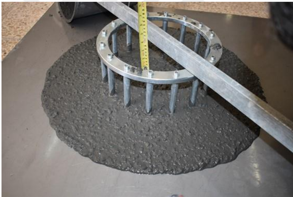
Figure 3.8. J-ring flow test: (a) schematically representation of equipment and (b) typical height difference measurement
