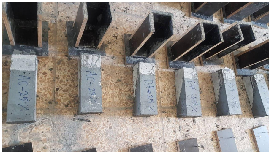
Figure 3.18. Slant shear strength test specimens including both old and new concretes
