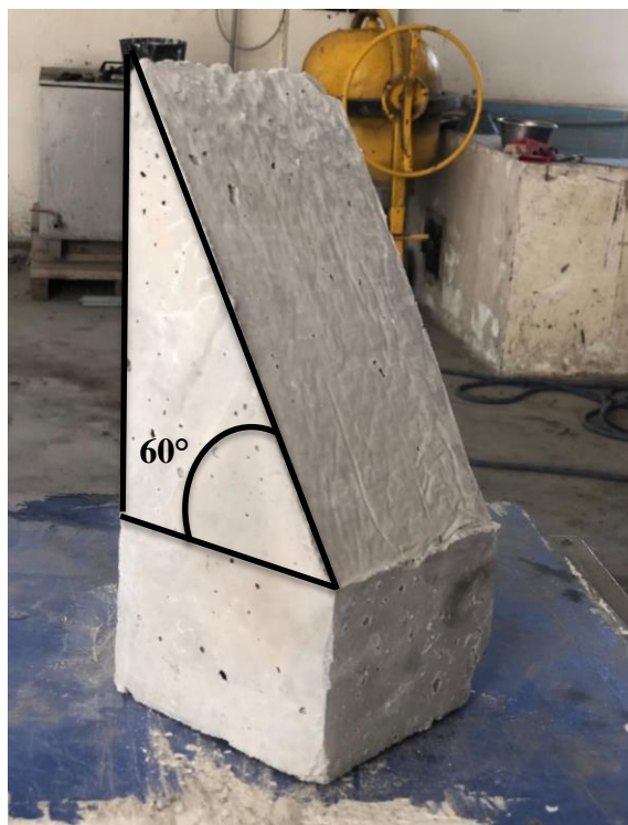
Figure 3.10. A typical ordinary concrete part of slant shear strength test
