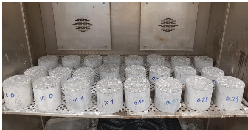
Figure 3.19. Sorptivity test specimens in the oven
