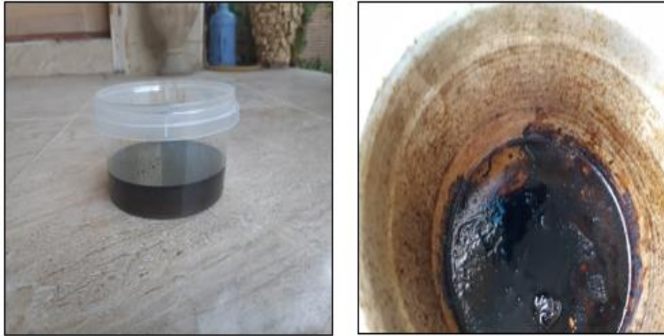
Figure 4.8 Oily wastewater before and after drying in the oven for 24 hours.
