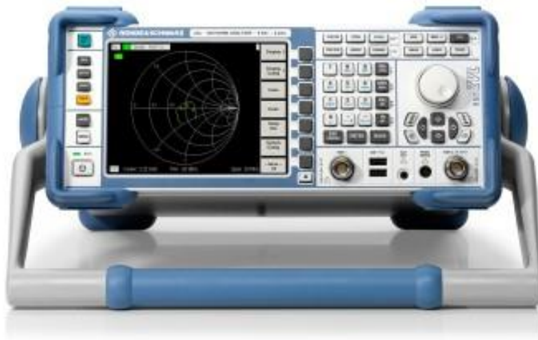
Figure 3.3. The Vector Network Analyzer Rohde & Schwarz ® ZVL13 with frequency range of (9 kHz ~ 13.6 GHz).
