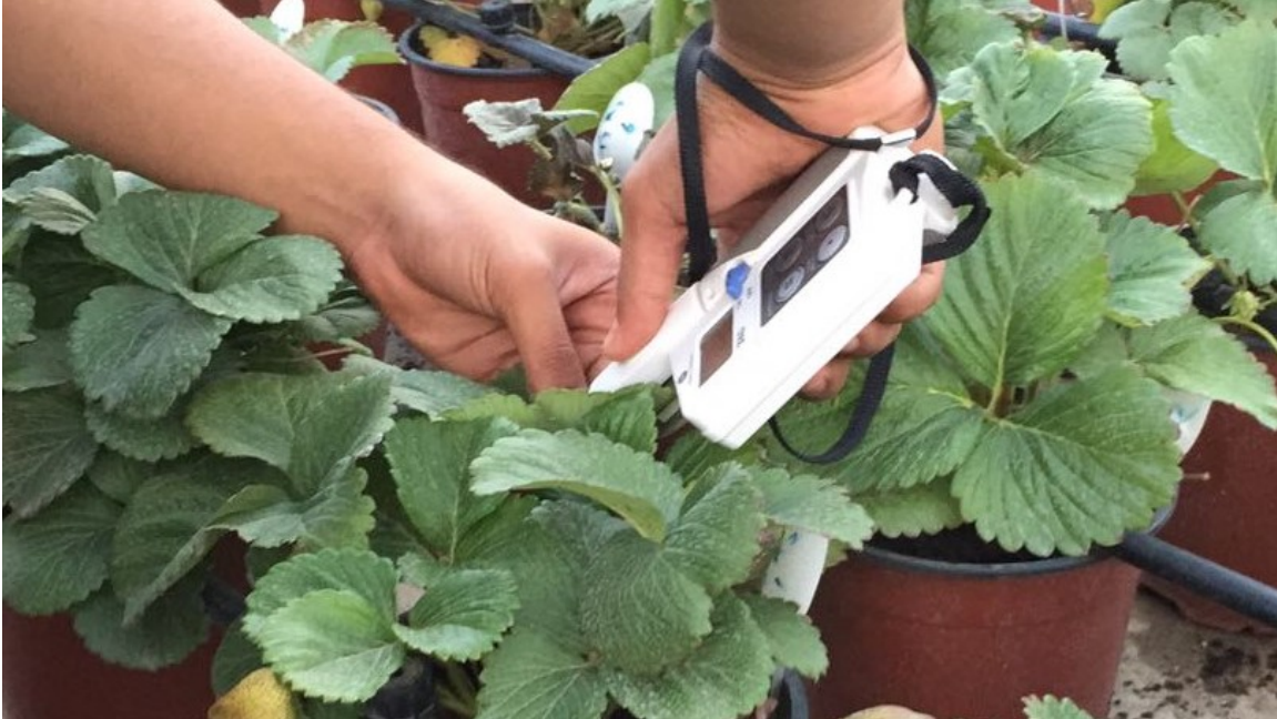
Figure 3.25. When using a chlorophyll measurements device (Konica Minolta SPAD-502 plus).
