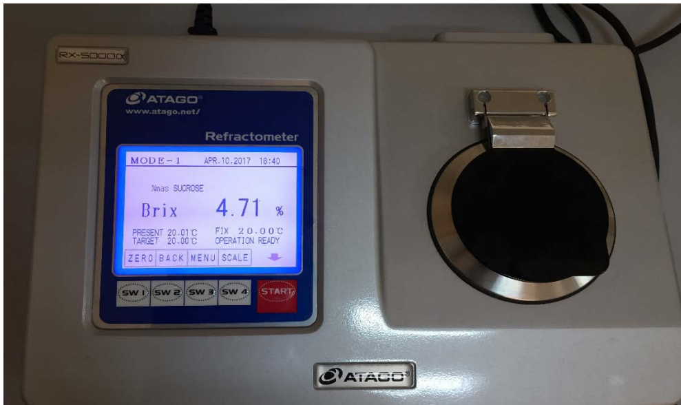
Figure 3.29. Table Refractometer (Atago Automatic Digital Refractometer, RX-5000).
