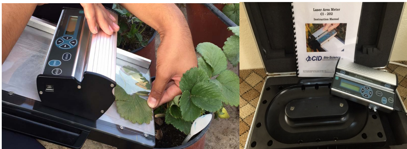
Figure 3.24. CI-202 portable laser leaf area meter, that used for measuring leaf area.
