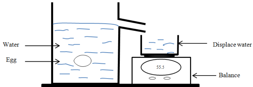
Figure 3.1. Archimedes principles of the egg volume measurement
