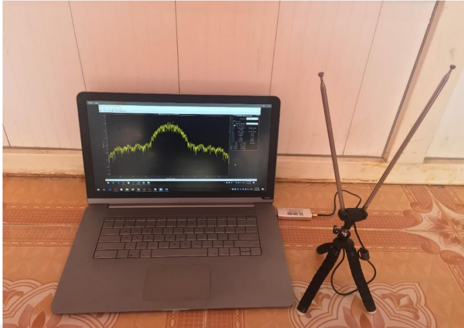
Fig 3.3 Host Vizio laptop, RTL-SDR and communication software
