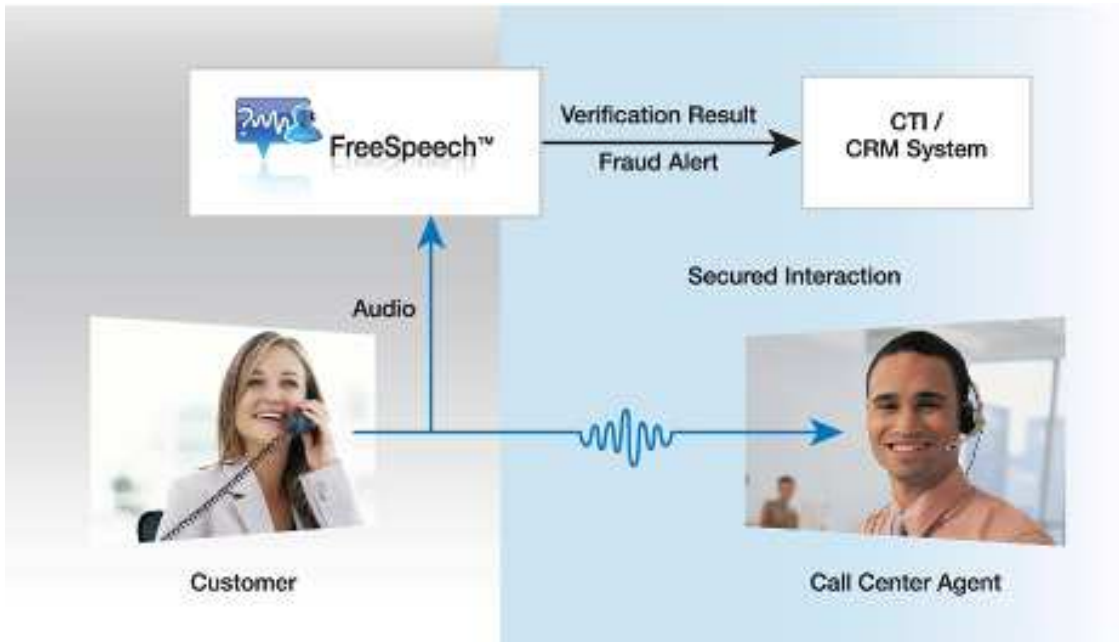
Figure 4: Automatic verification system aided call center scenario. The agent asks certain number of questions according to the score returned by the system. No additive effort needed for the agent, scoring is done during the flow of natural conversation.
