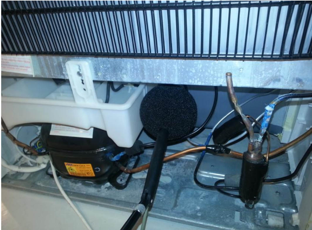
Figure 4.6 Microphone position in pressure measurement
