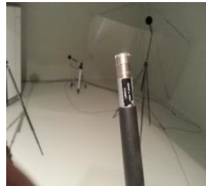
Figure 4.2 The 1/2-inch diffuse field microphone that is used in measurement
