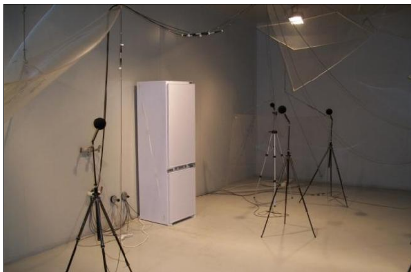
Figure 4.5 Reverberation chamber where measurement is done
