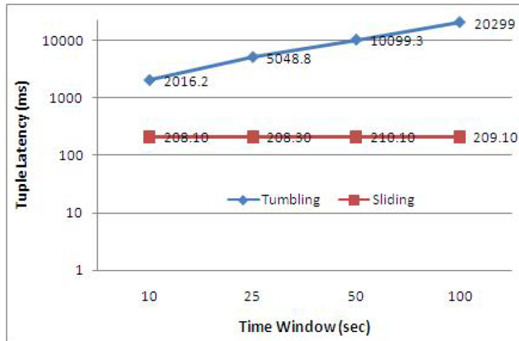
Figure 7: Performance comparison of sliding and tumbling windows at different window sizes.
