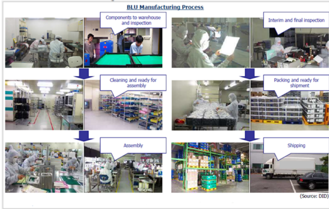
Figure 24: back light Unit Manufacturing Process [9]
