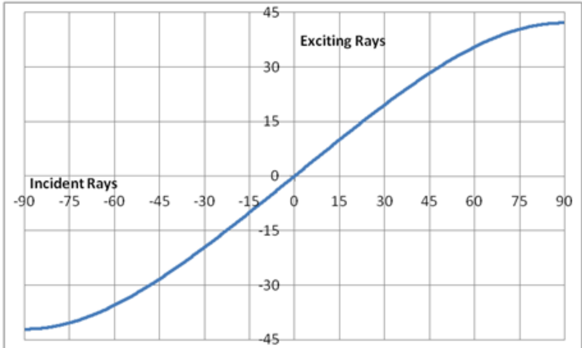
Figure 111: Snell's Law on PMMA - Air Interface
