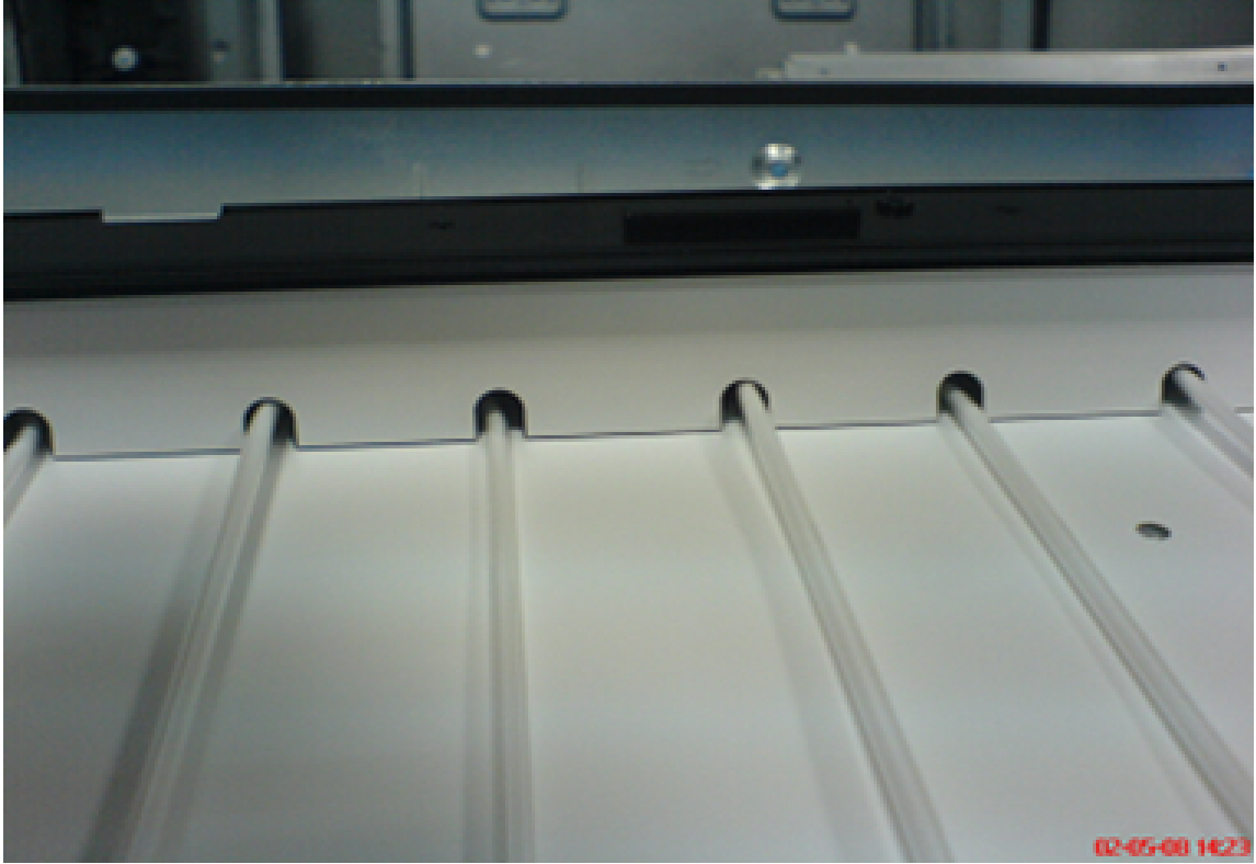
Figure 20: CCLF Based back light Unit [2]
