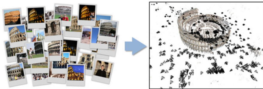
Figure 9: Bundler takes unordered image collections as inputs and outputs 3D map of the scene
