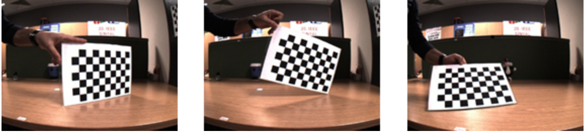
Figure 28: Sample frames used for camera calibration
