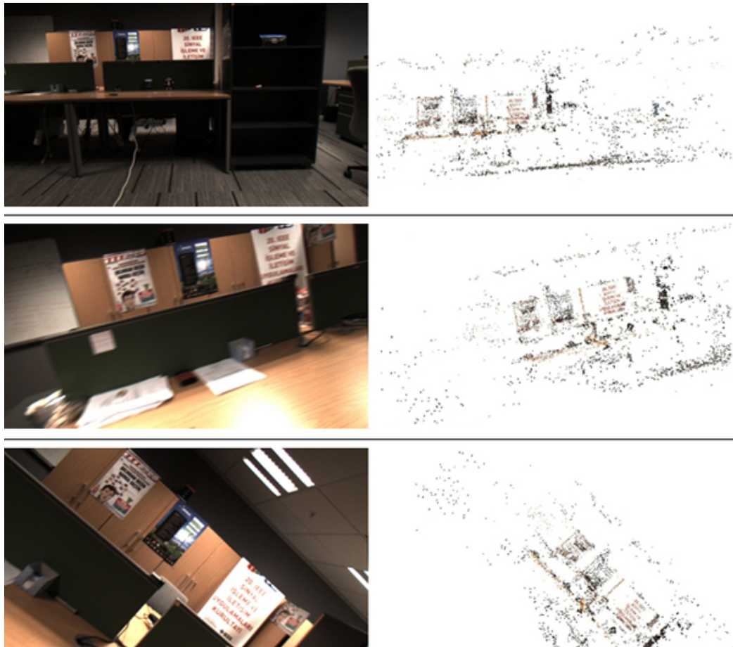
Figure 40: 3D point clouds viewed with respect to the camera pose of current frame
