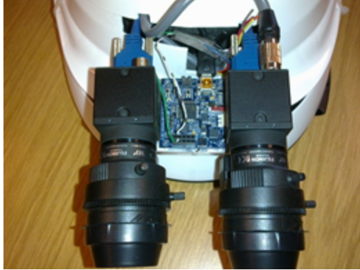
Figure 17: Camera and IMU combined on same media and mounted on an industrial safety helmet
