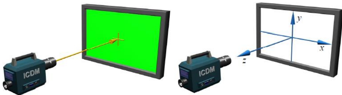
Figure 26: Optical measurement device setup for LCD TV
