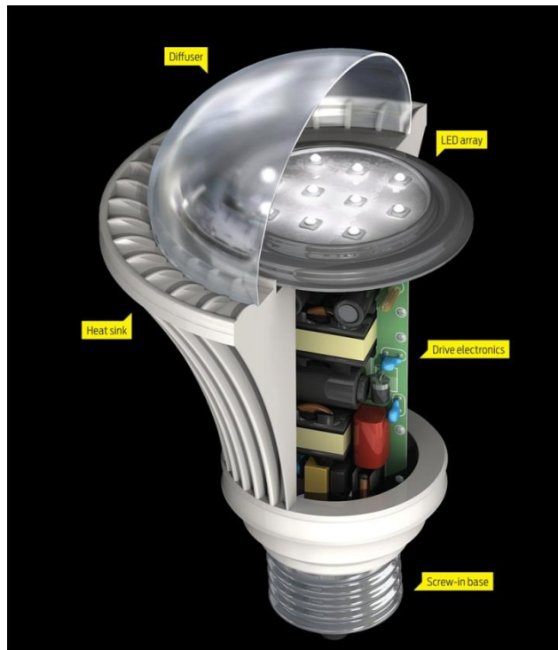
Figure 1: A typical LED lighting system with various components [1]
