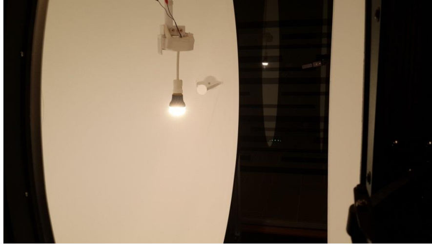
Figure 66: Optical test of prototype in integrating sphere
