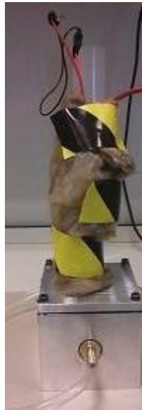
Figure 55. Experimental setup for heat pipe performance test
