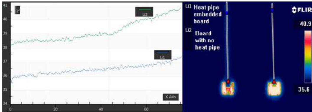
Figure 63. Comparison between a heat-pipe embedded in a plate using IR image (right); Line 1 representing a heat pipe embedded in board and Line 2 a simple heater on a simple board (no heat pipe)
