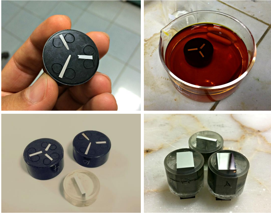
Figure 15: Optical macroscopic (OM) sample preparation for all tested conditions (E407) for grain structure under polarized light. A ZEISS optical microscope, Axio Imager A2 model, equipped with transmitted polarized-light bright field, with ergo-tube 20°/23 linked with a computerized imaging system (software) was employed for metallography observations.
