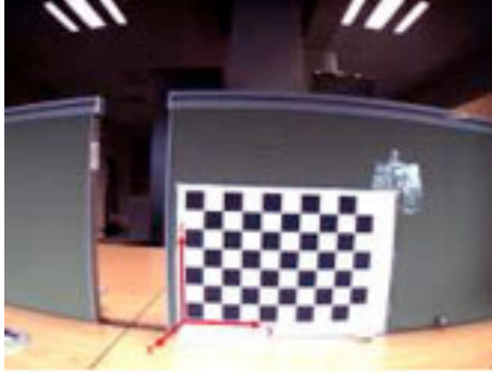
Figure 35: Gravity aligned calibration pattern.
