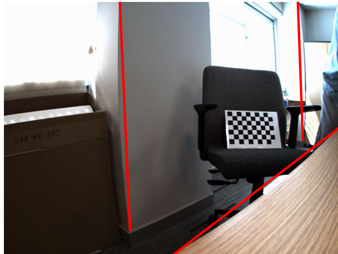
Figure 37: A image taken with a Point Grey Flea3 to show effects of distortions.
