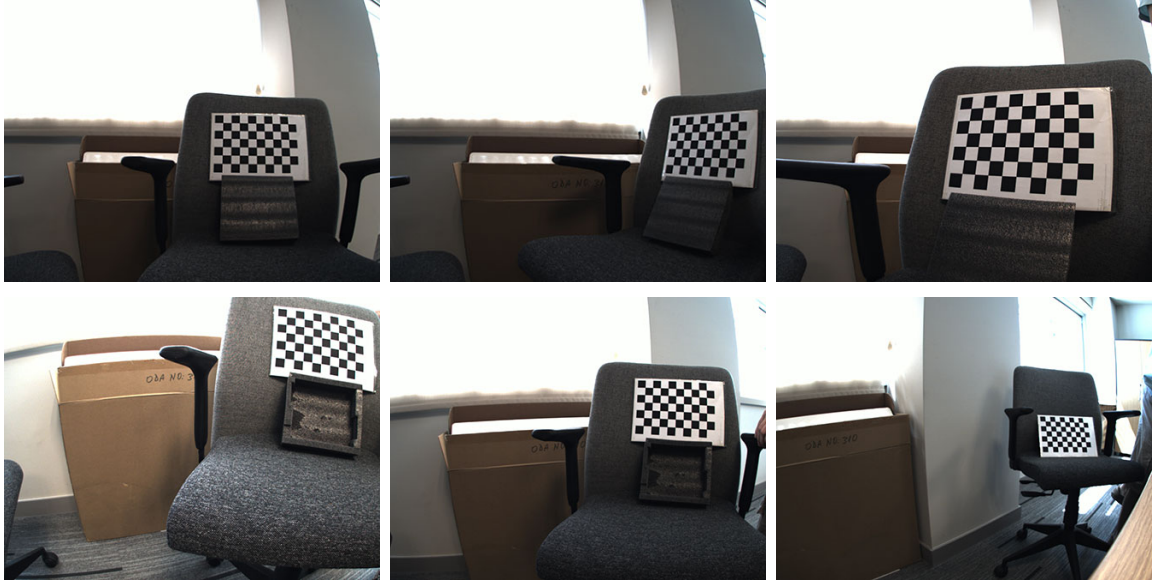
Figure 38: Mosaic of images used for camera calibration.
