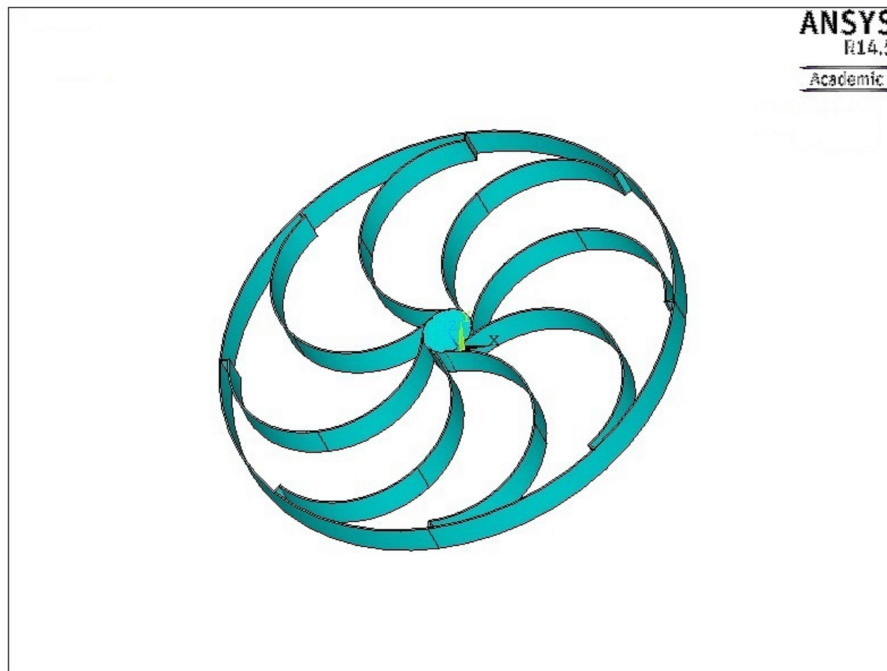
Figure 4.23: The HARPSS Vibrating Ring Gyroscope.
