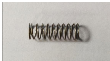
Figure 36. Picture of a coil spring made of 0.3mm stainless steel wire.
