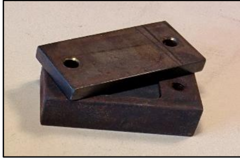
Figure 23. Picture of forming fixtures and their casing
