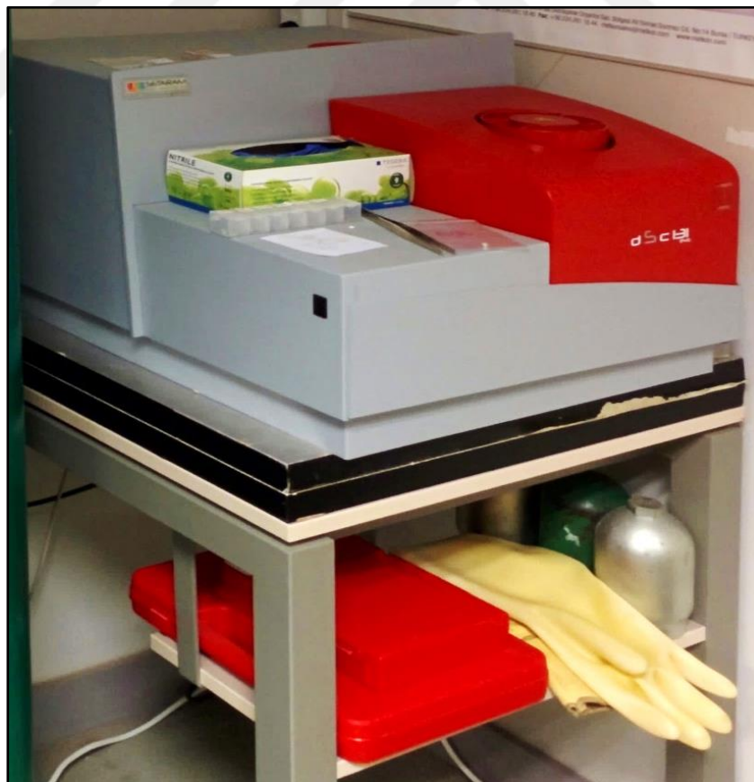
Figure 29. Picture of the DSC machine in the laboratory
