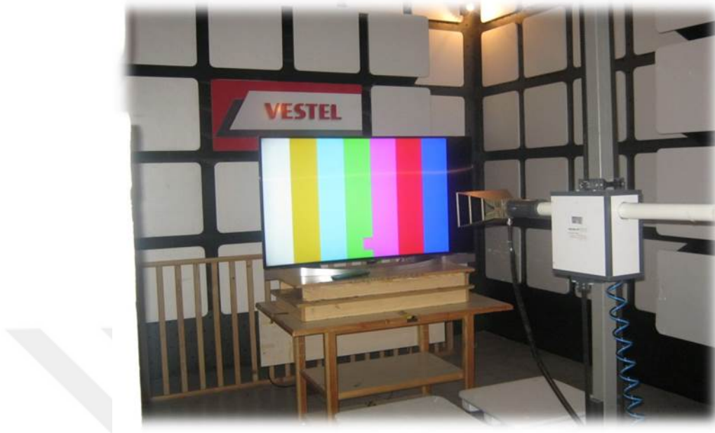
Figure 6: Example of effective radiated power test setup
