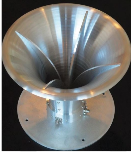
(a) Quad-ridged circular horn antenna [11] (b) A double-ridged rectangular horn [12]
