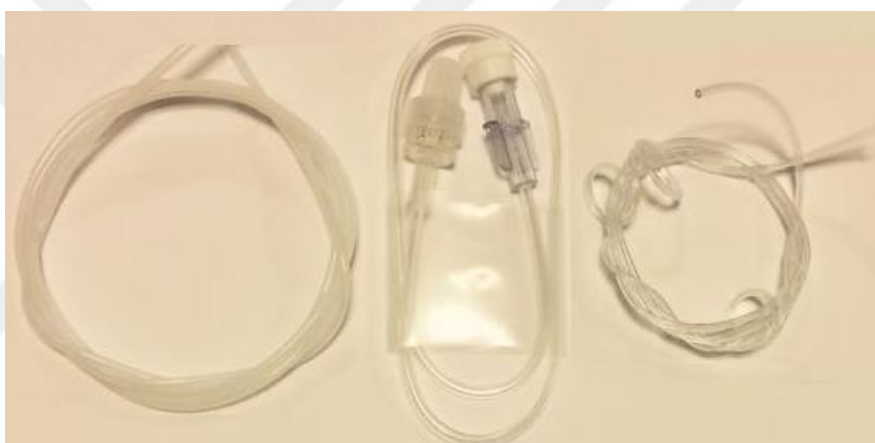
Figure 23. Tubing with different dimensions to find the suitable dimension for the flow-injection method
