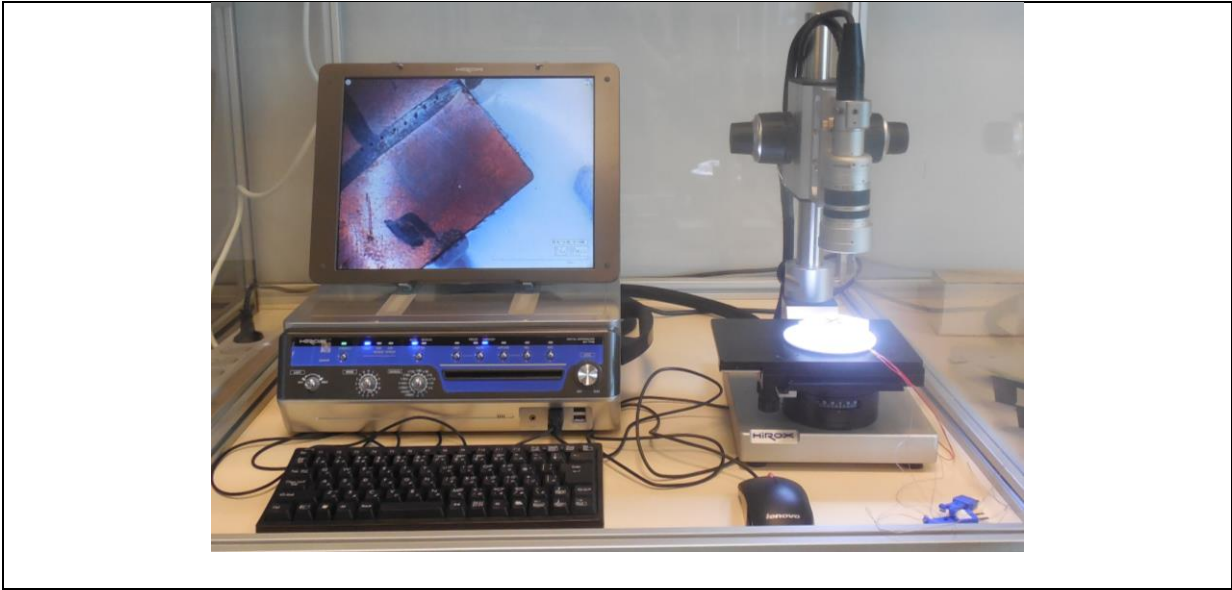
Figure 12: HIROX KH7700 microscope used for the heater surface evaluation
